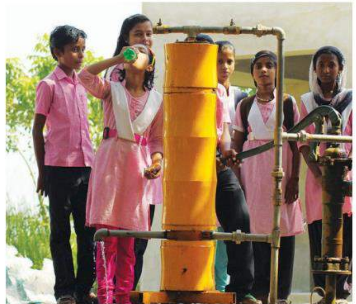
A water purification unit using nanomaterials connected to a handpump © Indian Institute of Technology, Madras
