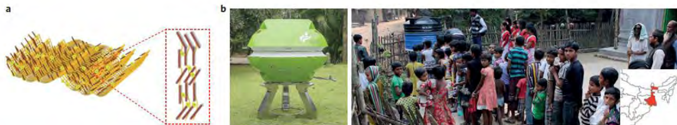
Figure 4 | Promising example of commercialized nanotechnology. a , A silver nanocomposite, Ag-BM, used for metal decontamination of water, formed from silver nanoparticles (yellow spheres) embedded in a matrix of alumina (brown rods) templated on chitosan fibrils (ochre filaments). b , A resulting product for arsenic and metal decontamination of water named AMRIT, undergoing installation in the arsenic- and iron-affected regions of the Murshidabad District, West Bengal (inset), and currently serving 30,000 people. The technology has resulted in the incubation of the Indian Institute of Technology Chennai-based company InnoNano Research. Panel a adapted with permission from ref. 11, © 2013 NAS. Inset, © Daniel Kaesler/Alamy.
